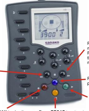
Press **FF** to fast-forward the master and student track. Press twice to go directly to the end. Press during play mode to wind forward slowly.
